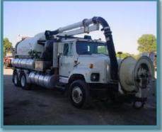
**Vactor Truck** – The Utility Department took delivery of a new Vactor Truck in July 2015 and put it into service for the fall lift station cleaning and the 2015 rodding schedule. The Maintenance department was able to use the vactor truck in maintaining the storm drain system. Nearly a third of the storm drains were vactored this year and another third of the system will be vactored each year.
